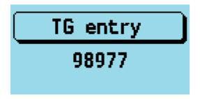
When a TG has been manually entered, the display shows a 1 pixel box around the TG display area to indicate that this TG has been manually entered, even if the Contact / TG name is displayed rather than the TG number.
