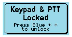
You can also lock the PTT button by pressing the **Green** menu key to display the Main menu and then pressing the **Hash (#)** key. The keypad *and* the PTT can both be locked at the same time by first locking the PTT and then the keypad.
