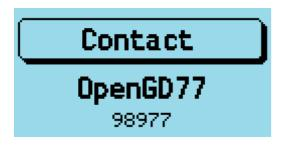
The contact name is show in the middle of the screen, e.g. "TG 505 TS2" and the TalkGroup or PC number is shown in smaller text at the bottom of the screen.
