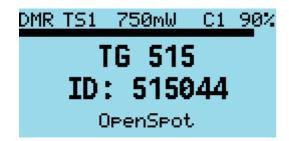
If the DMR ID is in the DMR ID database previously loaded into the radio, the callsign and name will be displayed.
