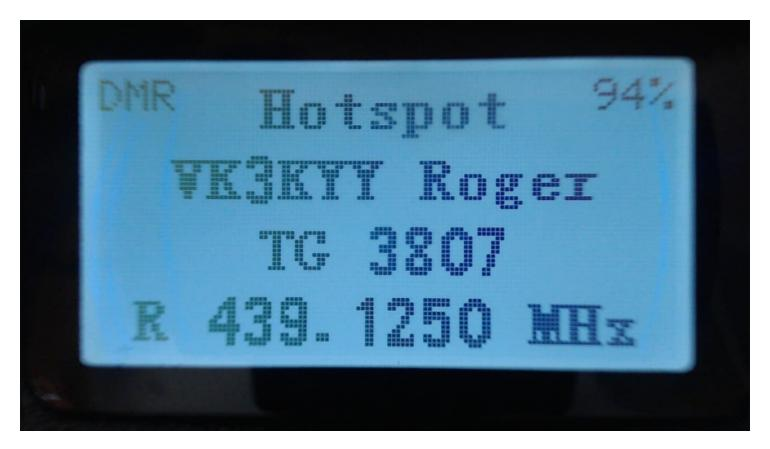
When PiStar receives traffic from the Internet and sends it to the hotspot for transmission, the hotspot displays the Callsign and name or the DMR ID, and the TX frequency is show.
