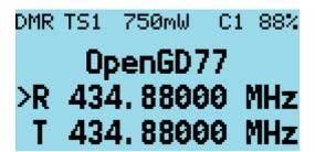
The VFO displays both the TX and RX frequency at all times.
