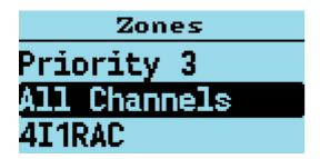
When the All Channels zone is selected, the Channel screen displays the "**All Channels** and the channel number instead of the zone name and channel number.
