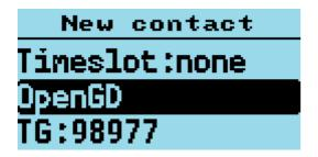
Press **Left** and **Right** to move the cursor. Press **Function-Left** as backspace, and **Function-Right** to insert a space. The keypad entry follows the same functionality as stock GD77 firmware.
