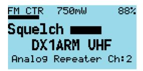
Once in squelch control mode, pressing **Right** tightens the squelch incrementally, **Left** opens up the squelch incrementally. The VFO and each channel have individual squelch settings that can be set in this manner.
