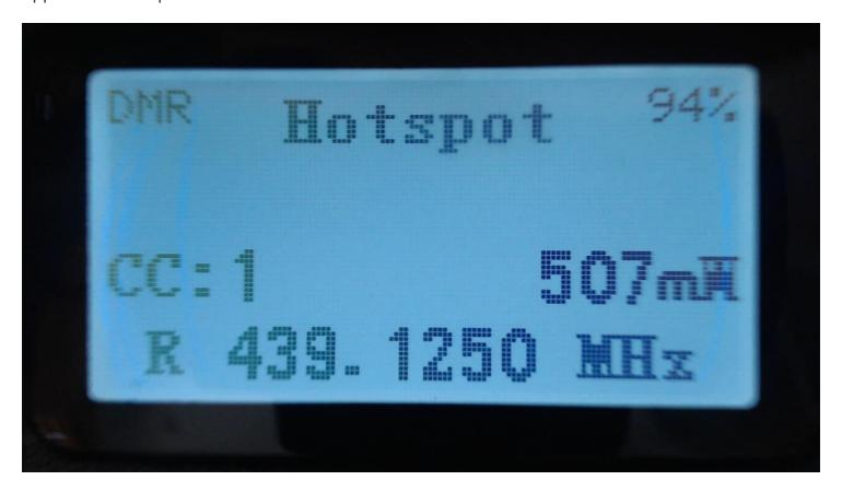
If the radio does not enter Hotspot mode, power cycle the radio and power cycle PiStar If the radio still fails to enter hotspot mode, check your USB connections.
