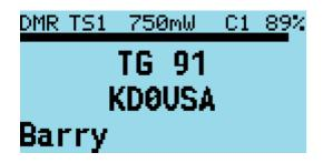
Note: As the Talker Alias data is sent slowly as it is embedded inside the DMR audio data frames, the callsign will appear first and about half a second later the DMR ID or other text will arrive via the DMR data and be displayed.
