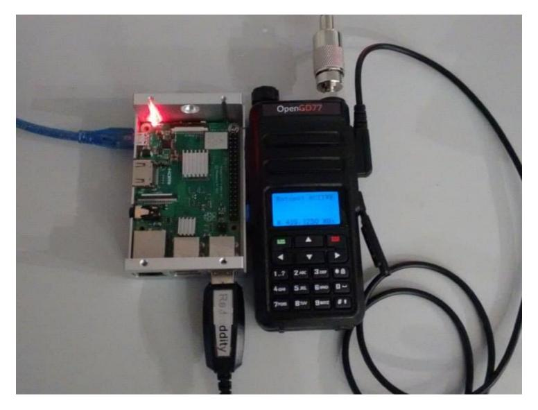
Hotspot mode works with the Raspberry Pi Zero, but a adaptor cable is needed to convert from the micro USB port on the RPi Zero to the full size USB plug on the radio's programming cable.
