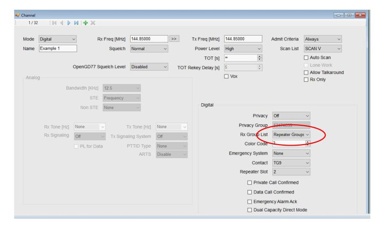
*Note.* The "Contact" is not used by the firmware. You must use the TG list to define the TG's you want to use with each channel. Hence you must have at least 1 TG list and it must contain at least 1 Digital Contact which is a TalkGroup.
