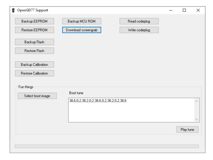
From here you can backup, the internal 64k EEPOM and the 1 mega byte Flash chip, as well as Reading and Writing the codeplug. The calibration data store in the Flash chip (At address 0x8f000) can be backed up and restored without backing up the whole of the Flash.
