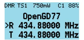
The frequency used in the VFO for both Tx and Rx will be read from the "VFO A" settings of the codeplug.
