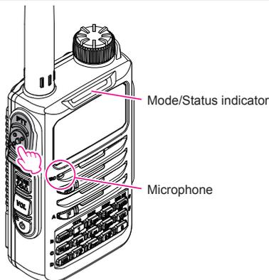
2. Release the **PTT** switch to return to receive mode.
